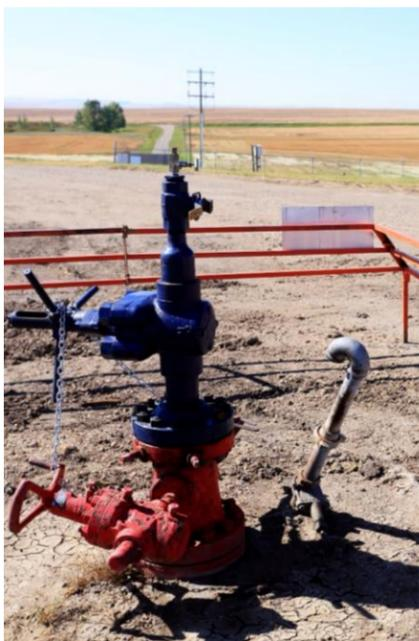
Well head with casing vent
